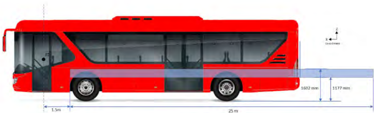
Figure 19_14: Side view of wide-angle assessment zone
